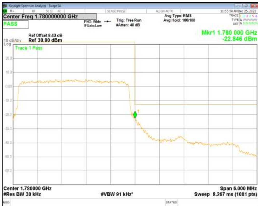
Band66 QPSK BW=5MHz Channel=131997 RB Size=25 Position=#0
