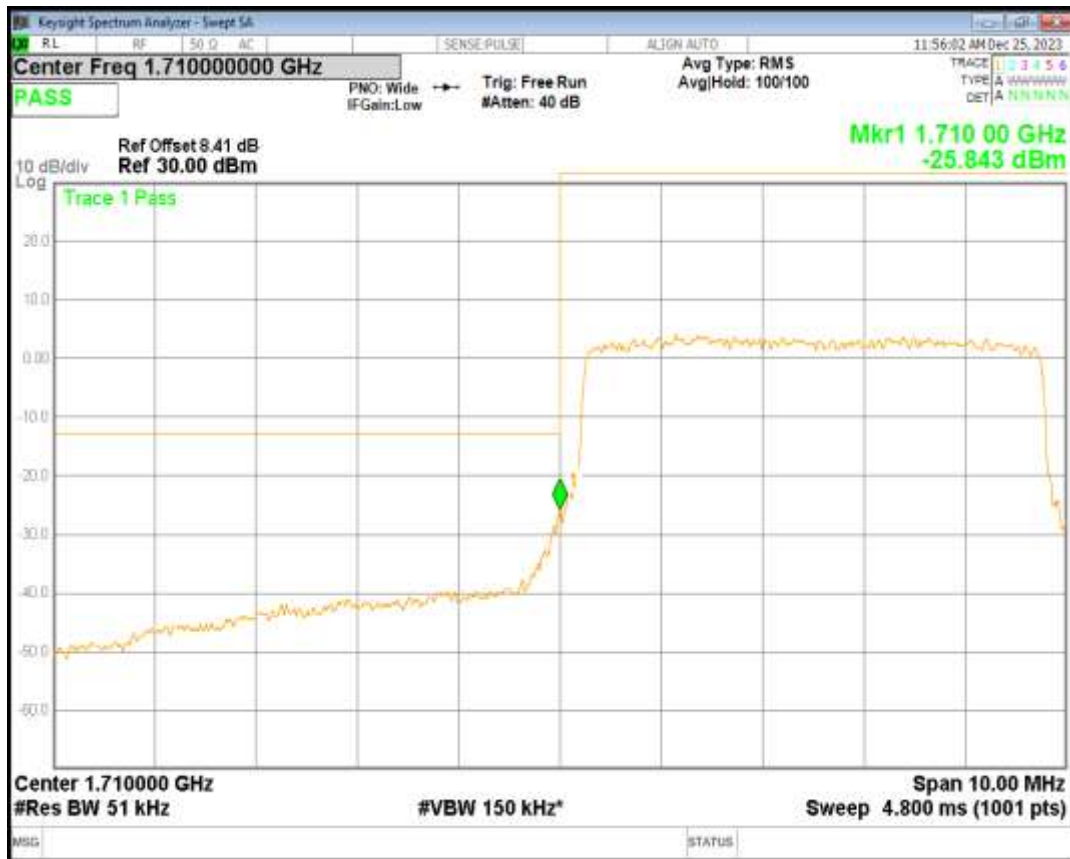
Band66 16QAM BW=5MHz Channel=132647 RB Size=25 Position=#0
