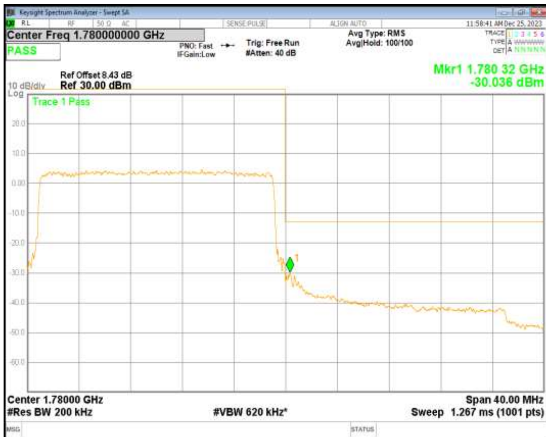
Band66 QPSK BW=3MHz Channel=131987 RB Size=15 Position=#0
