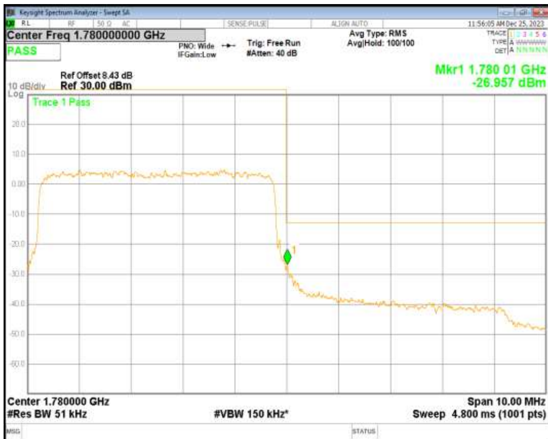
Band7 16QAM BW=5MHz Channel=20775 RB Size=25 Position=#0
