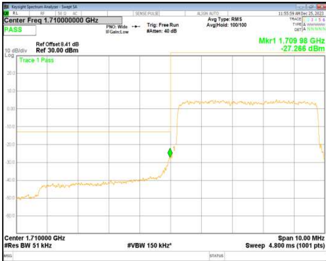
Band66 QPSK BW=5MHz Channel=132647 RB Size=25 Position=#0
