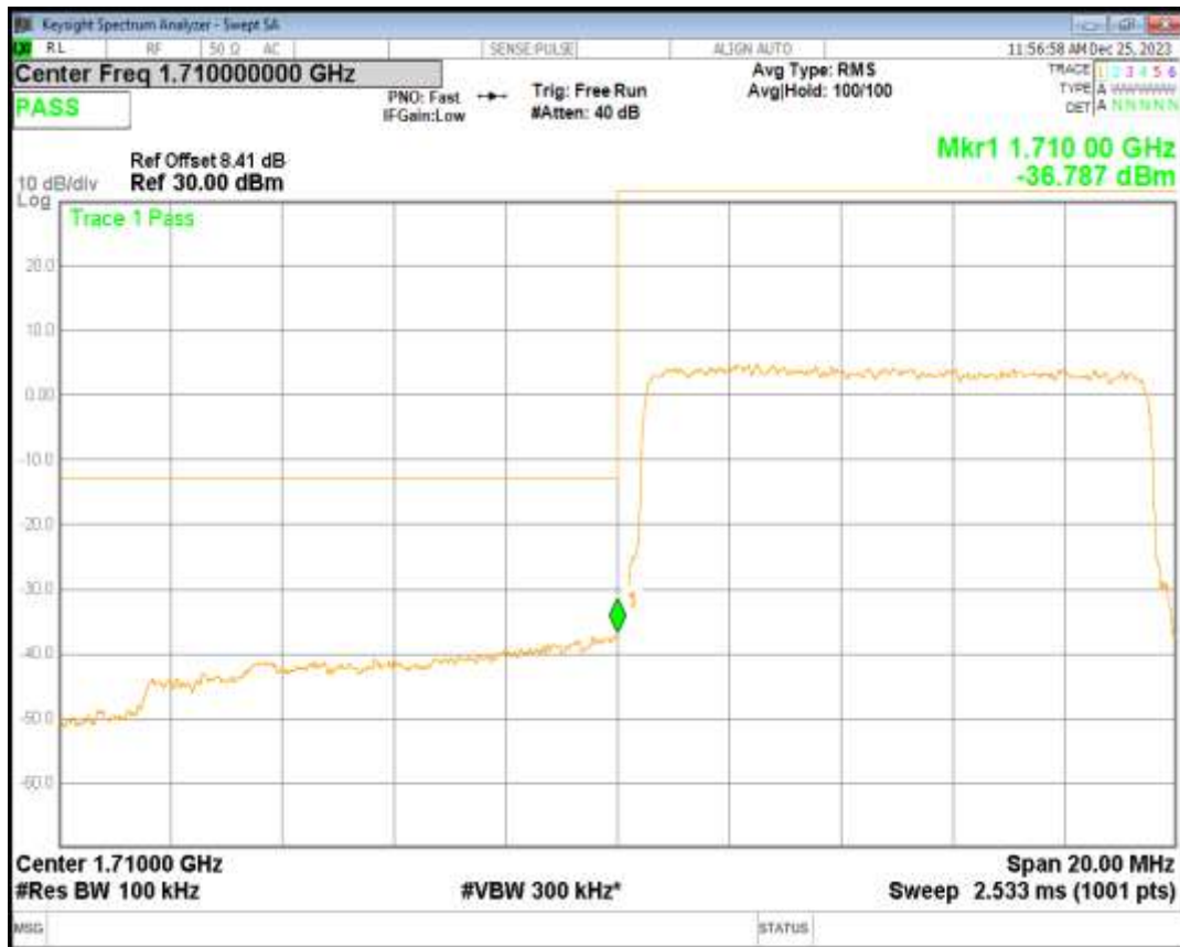
Band66 QPSK BW=10MHz Channel=132622 RB Size=50 Position=#0
