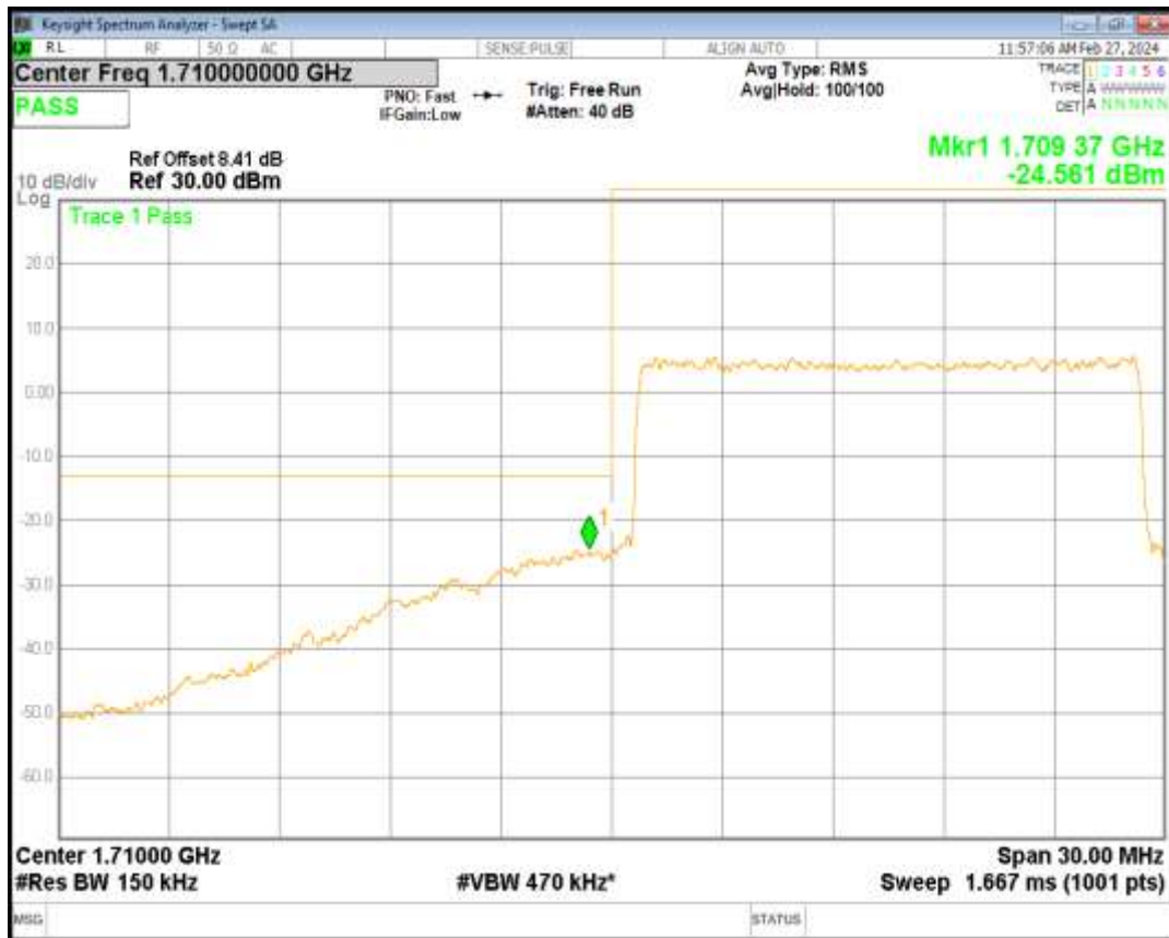
Band66 QPSK BW=15MHz Channel=132597 RB Size=75 Position=#0
