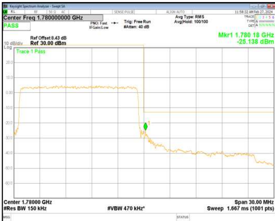
Band66 QPSK BW=20MHz Channel=132072 RB Size=100 Position=#0
