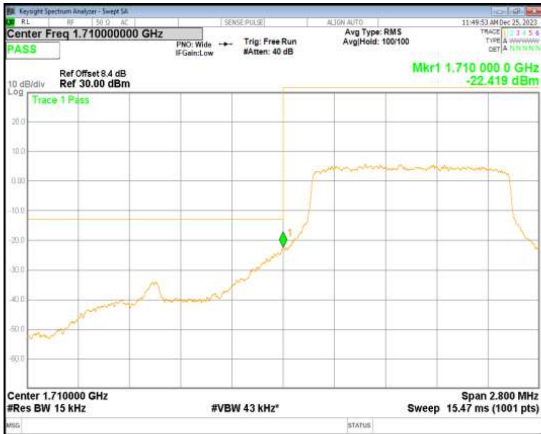
Band66 QPSK BW=1.4MHz Channel=132665 RB Size=6 Position=#0
