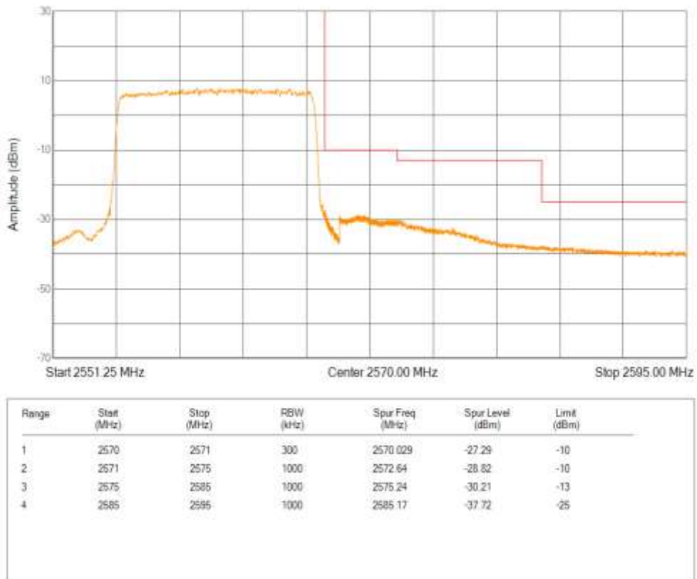
Band7 QPSK BW=20MHz Channel=20850 RB Size=100 Position=#0
