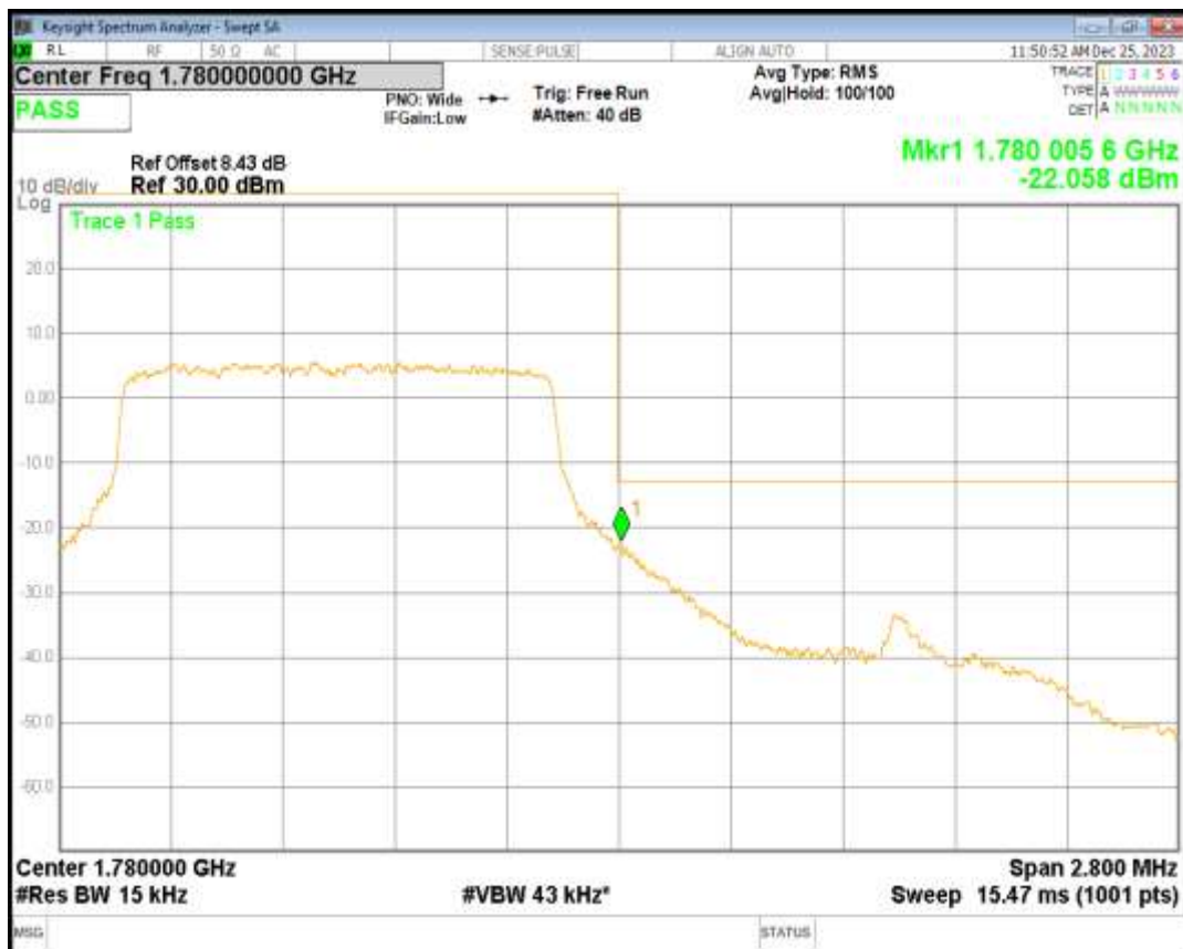
Band66 QPSK BW=10MHz Channel=132022 RB Size=50 Position=#0
