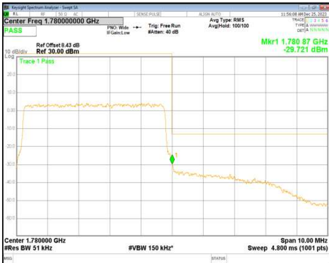
Band66 QPSK BW=1.4MHz Channel=131979 RB Size=6 Position=#0
