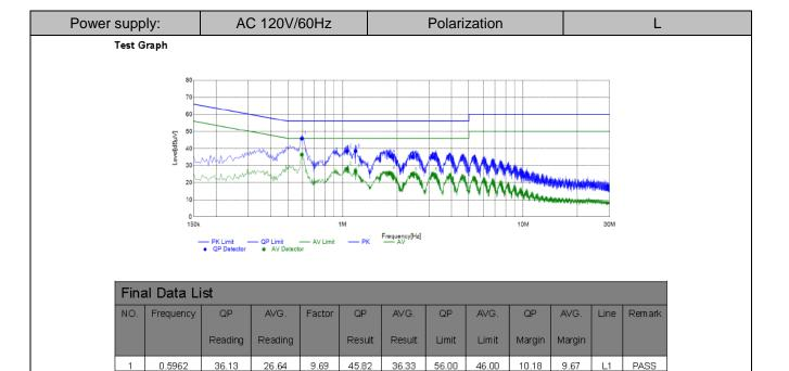
Note: 1. Result (dB $\mu$ V) = Reading (dB $\mu$ V) + Factor (dB).
