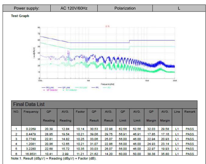
2. Factor (dB) = Cable loss (dB) + LISN Factor (dB).
