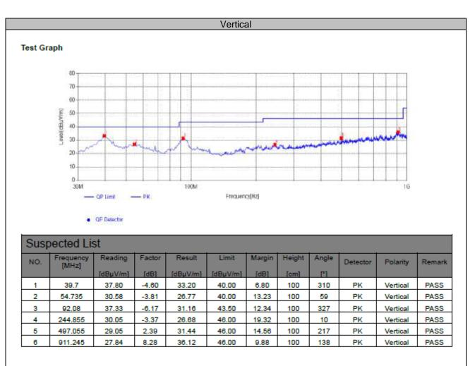
Note:1. Result (dBµV/m) = Reading(dBµV/m) + Factor (dB).
