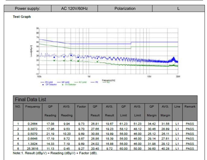
2. Factor (dB) = Cable loss (dB) + LISN Factor (dB).
