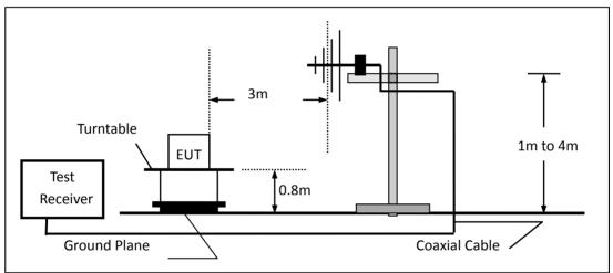
(c) For radiated emissions above 1000MHz
