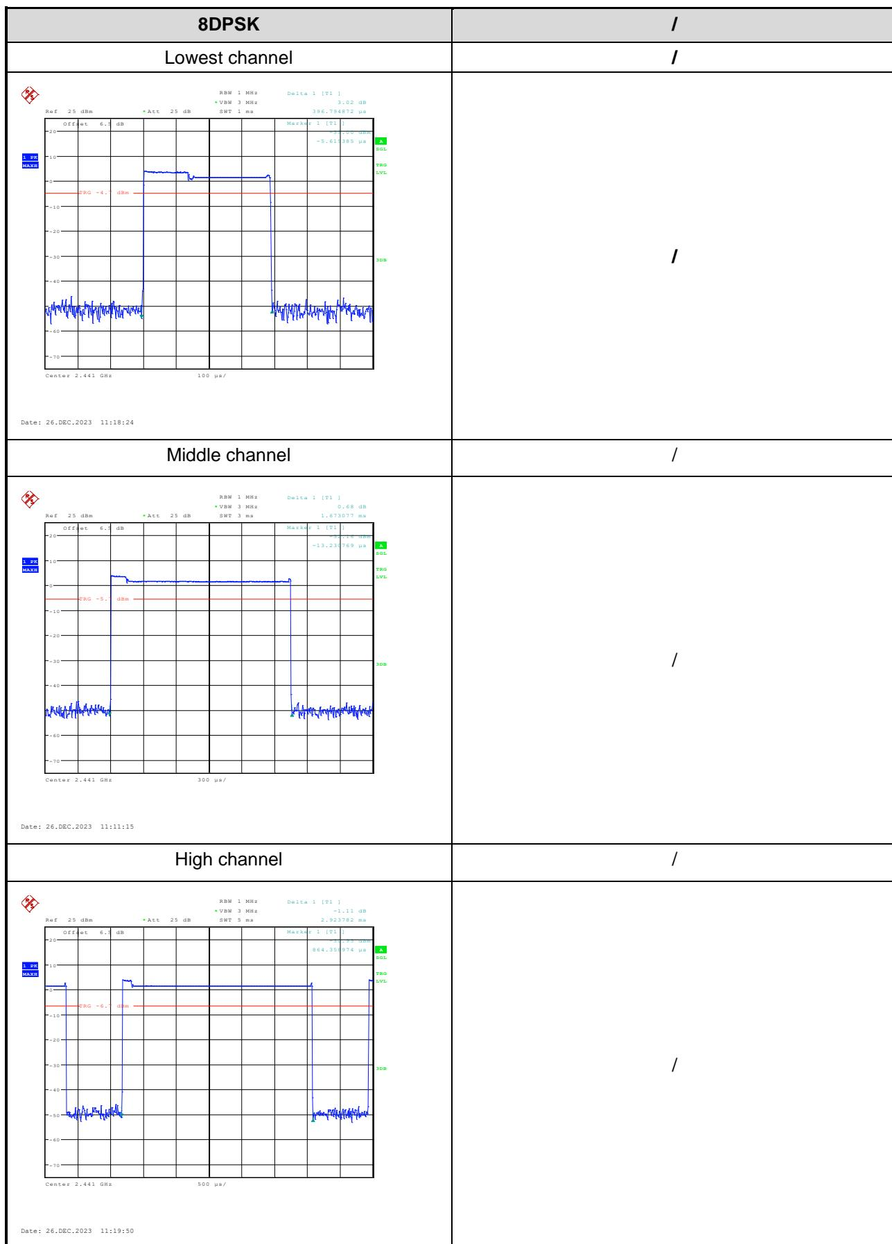
100kHz Bandwidth of Frequency Band Edge:
