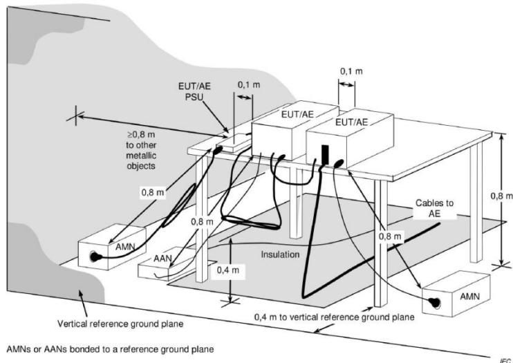
**Note:** The 0.8 m distance specified between EUT/AE/PSU and AMN/AAN, is applicable only to the EUT being measured. If the device is AE then it shall be >0.8 m.
