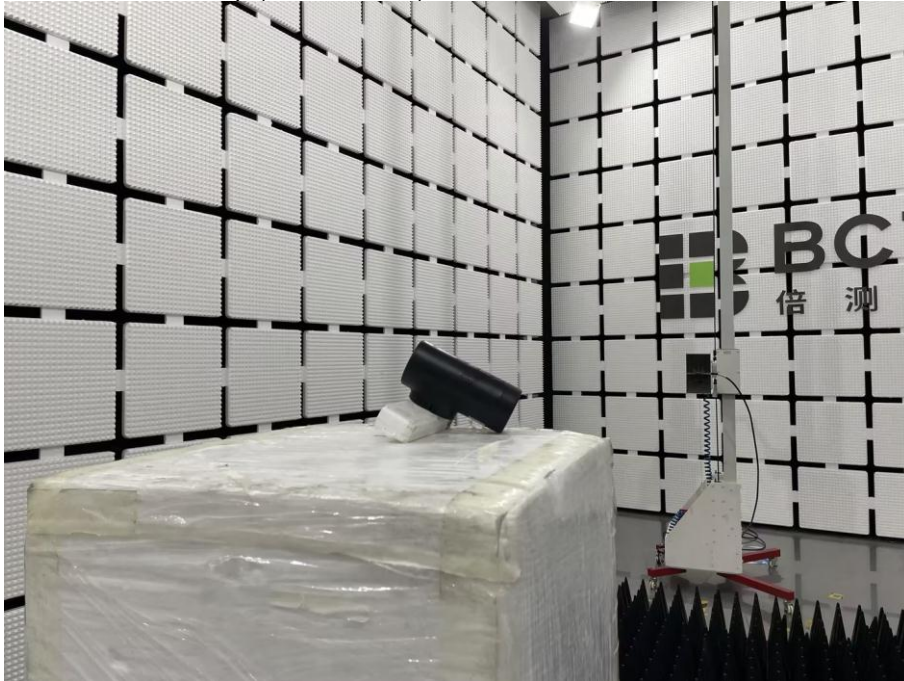
Spurious Emission Test Setup (Above 1GHz)
