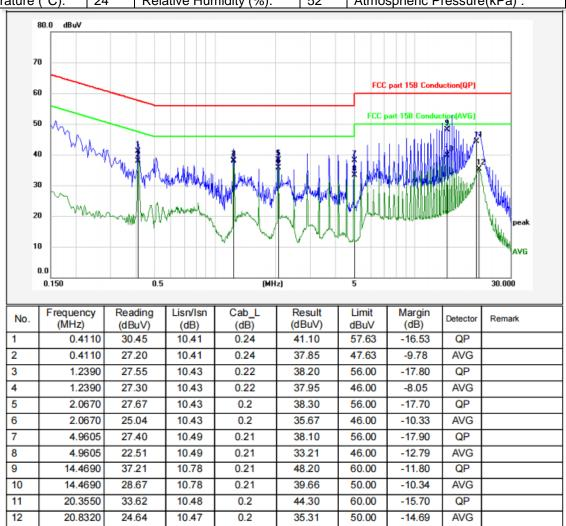
Remarks: 1. Result=Reading+Lisn+Cab\_L 2. If the average limit is met when using a quasi-peak detector. the EUT shall be deemed to meet both limits and measurement with average detector is unnecessary.
