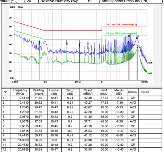
Remarks: 1. Result=Reading+Lisn+Cab\_L 2. If the average limit is met when using a quasi-peak detector. the EUT shall be deemed to meet both limits and measurement with average detector is unnecessary.
