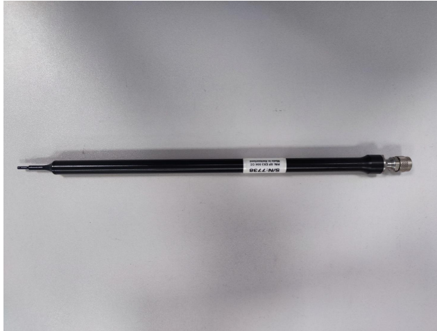
Figure 1-Speag COMOSAR Dosimetric E field Dipole
