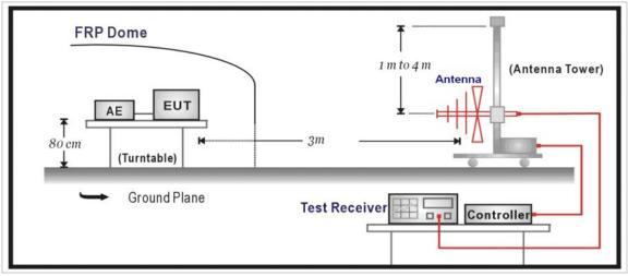
Above 1GHz Test Setup:
