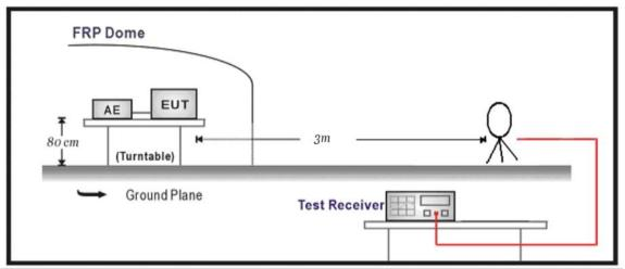
Below 1GHz Test Setup:
