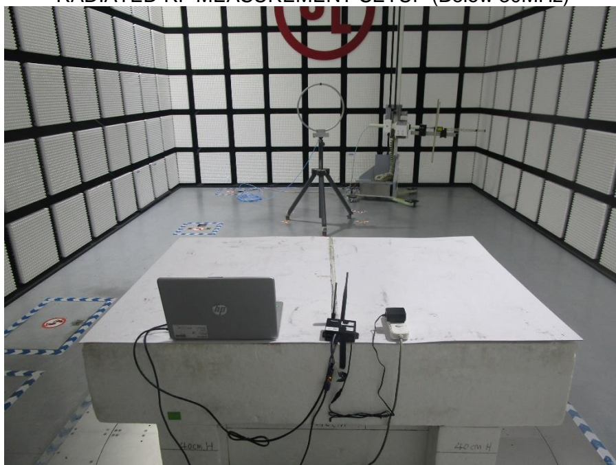
RADIATED RF MEASUREMENT SETUP (Below 30MHz)
