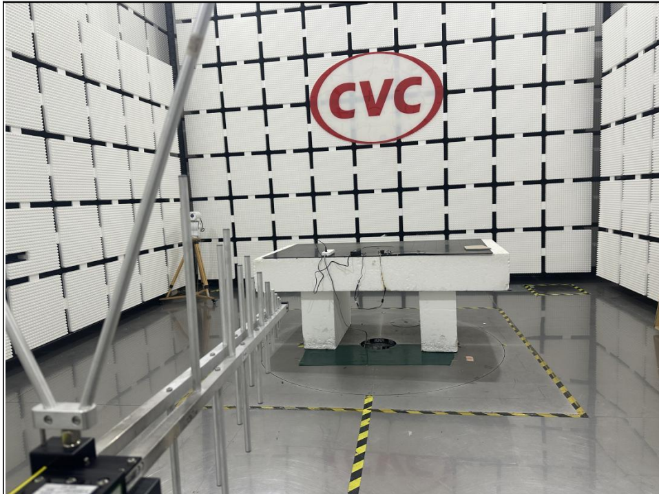
RADIATED EMISSION TEST (Below 1GHz)
