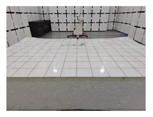
Set-up for Radiated Spurious Emission, Below 1GHz
