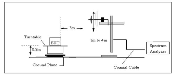
(C) Radiated Emission Test-Up Frequency Above 1GHz
