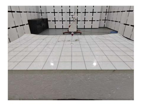
Set-up for Radiated Spurious Emission, Above 1GHz
