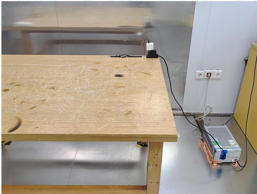
Photo of Setup for Conducted Emission
