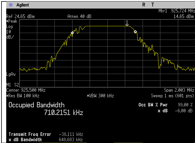
High Ch_925.5MHz_1MBit_Occupied Bandwidth_-6dB
