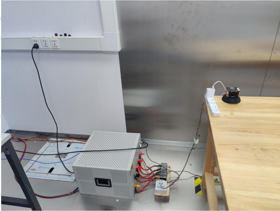
Photo of Conducted Emission Measurement
