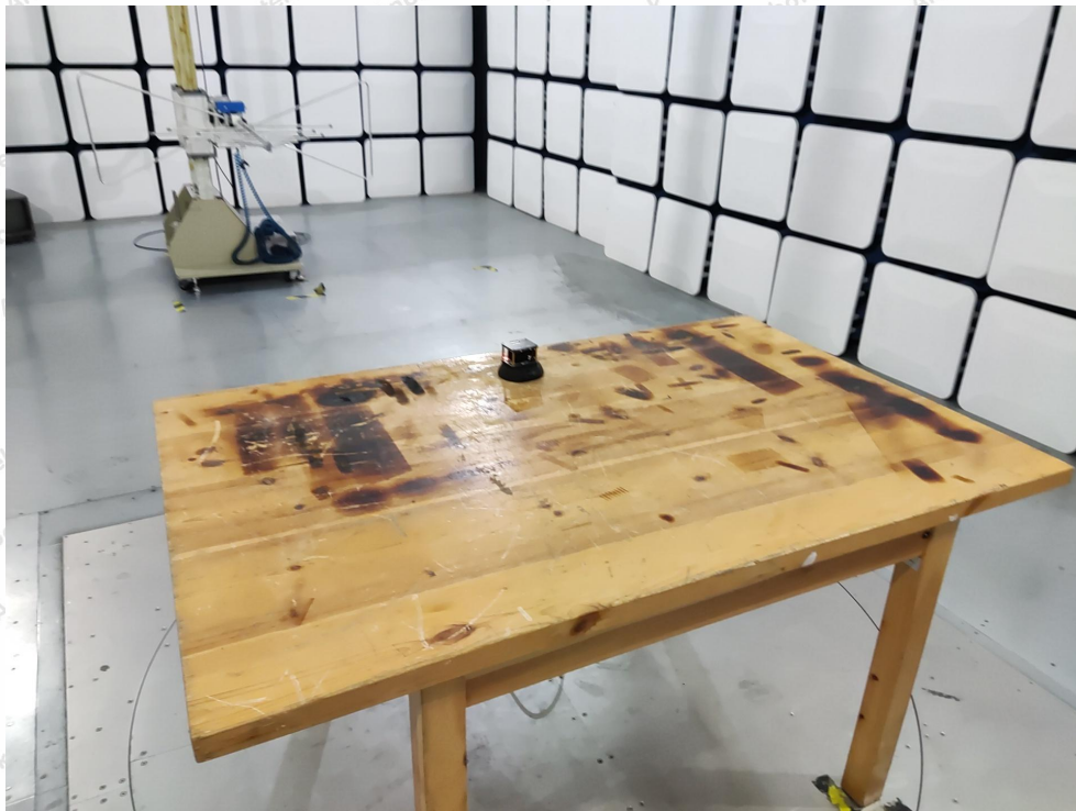
Photo of Radiation Emission Test
