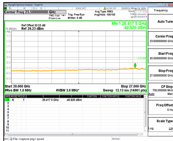
n41 (20GHz-27GHz) 40M DFT-s-OFDM BPSK Inner_1RB_Right Low
