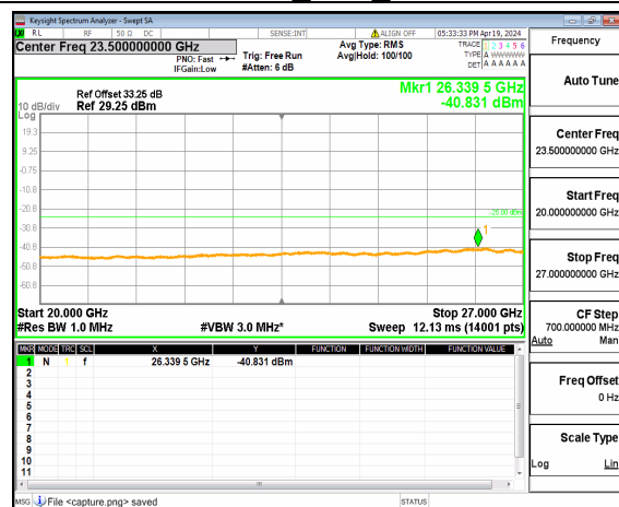
n41 (20GHz-27GHz) 80M DFT-s-OFDM BPSK Inner_1RB_Right Low
