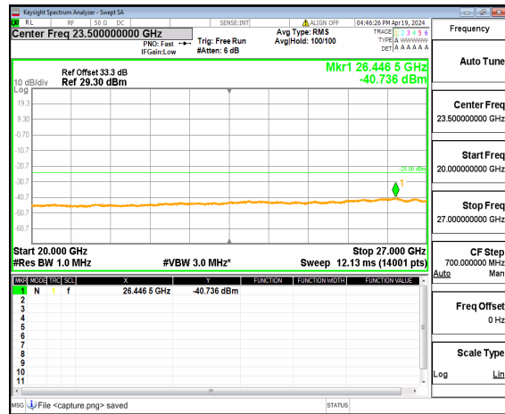
n41 (20GHz-27GHz) 50M DFT-s-OFDM QPSK Inner_1RB_Left Mid
