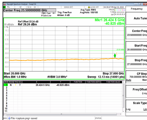
n41 (20GHz-27GHz) 50M DFT-s-OFDM BPSK Inner_1RB_Right_Low
