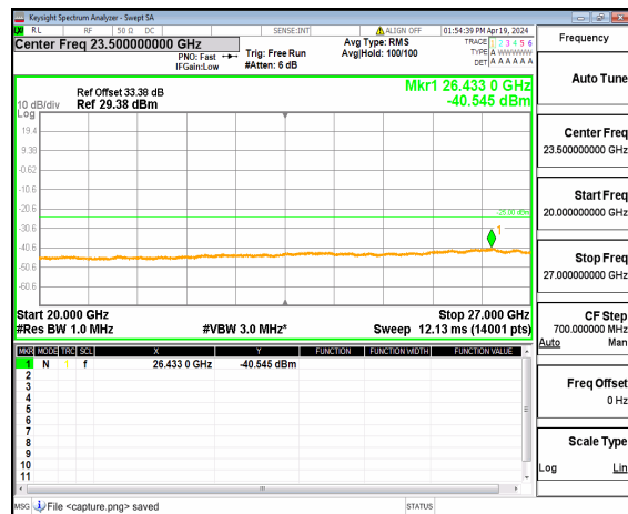
n41 (20GHz-27GHz) 30M DFT-s-OFDM QPSK Inner_1RB_Left_High
