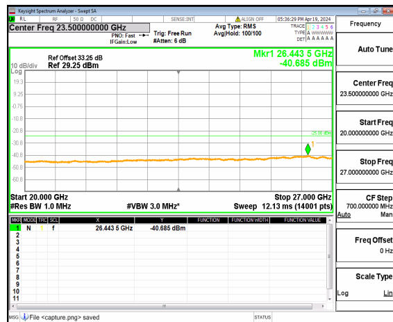
n41 (20GHz-27GHz) 80M DFT-s-OFDM QPSK Inner_1RB_Right Low
