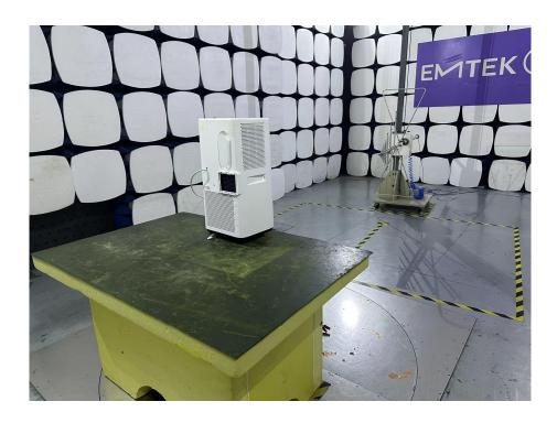
Spurious Emission Test Setup (Above 1GHz)
