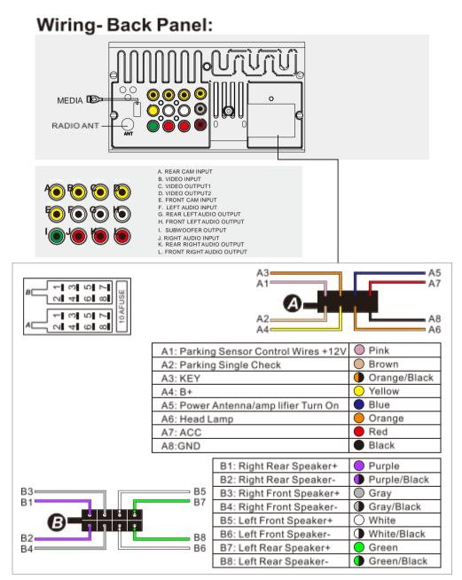
Please check the speaker line carefully before installation. If any grounding or touching, please connection again, otherwise the unit will be burned.
