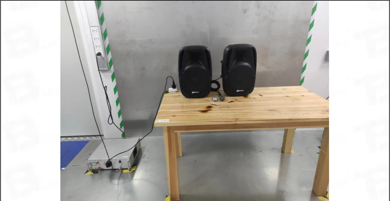
Conducted Emission at AC power line
