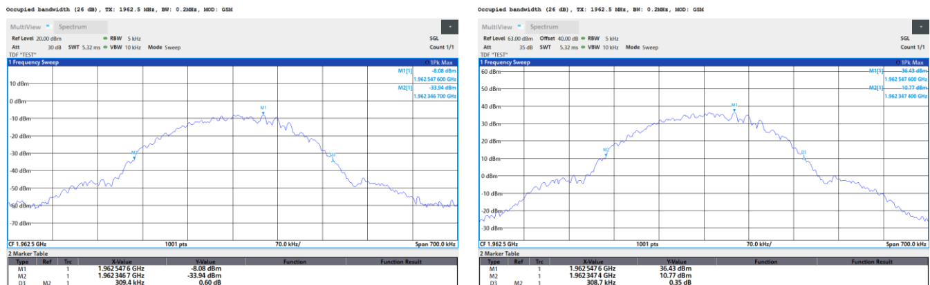
Figure 8.3-1: Occupied bandwidth / Input Versus Output Comparison results, narrowband signal, 0.5 dB below AGC threshold, input and output signal respectively
