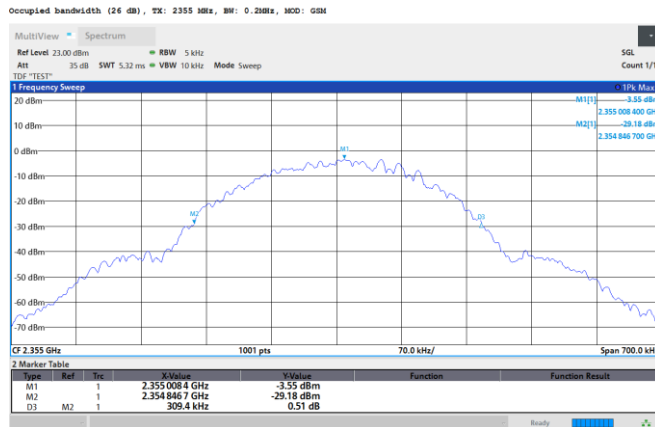
Figure 8.3-10: Occupied bandwidth / Input Versus Output Comparison results, narrowband signal, 3 dB above AGC threshold, input and output signal respectively
