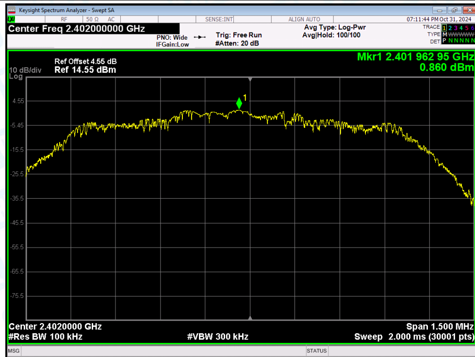
Tx. Spurious NVNT 3-DH1 2402MHz Ant1 Emission
