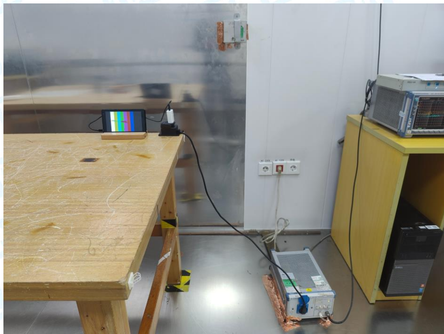
Photo of Setup for Conducted Emission
