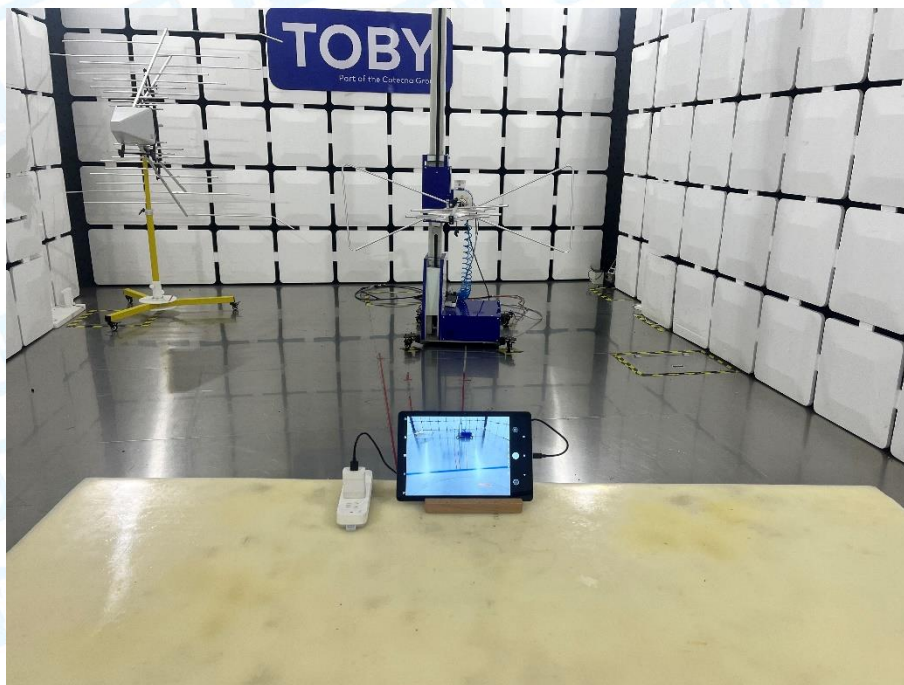
Photo of Setup for Radiated Emission (30MHz~1GHz)
