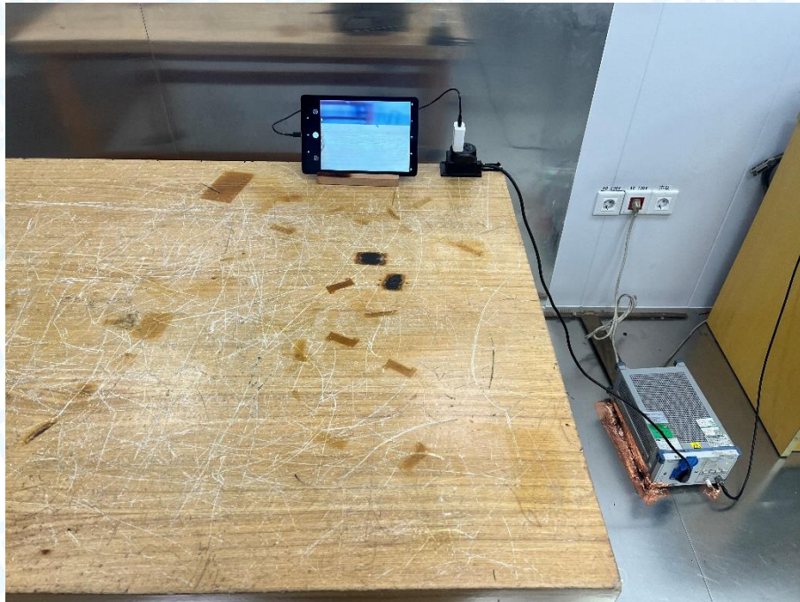
Photo of Setup for Radiated Emission (30MHz~1GHz)
