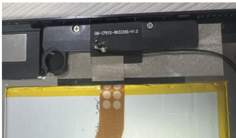
Here, the conductor cloth is attached to shield the flat cable below, and the copper leakage area of the antenna is grounded by the conductor cloth.
