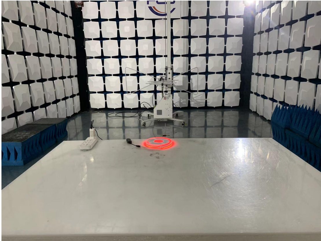
Above 1GHz for radiated emission test setup
