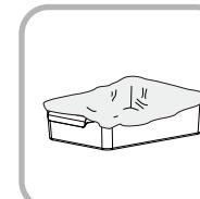
②. The garbage bag is first set to the rear two corners, and then pulled back and stuck on the front two clasps, and then smooth, reset the collection bin
