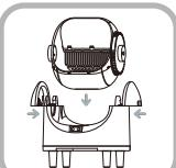
②. Place the machine on a hard and flat floor, install the drum first, and then press both sides of the handle inward by hand to install.
