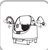
① Pull the handle outward from both sides to remove the handle
