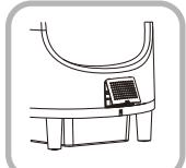
①. Find the cover plate on the side and press the two clasps on the cover plate, and then remove the cover plate.
