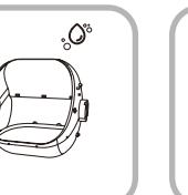
⑥ The rotary cylinder is cleaned directly with water
