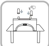
①. Take out the drum and other accessories, put the machine (as shown) upside down on the table, take out the four support legs and insert them into the corresponding positions in turn, put them to ensure the installation.
