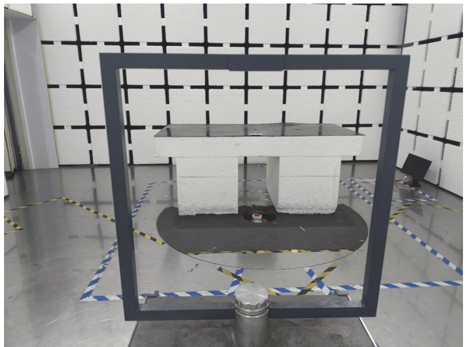
Radiation Emission Test Setup (Below 30MHz)
