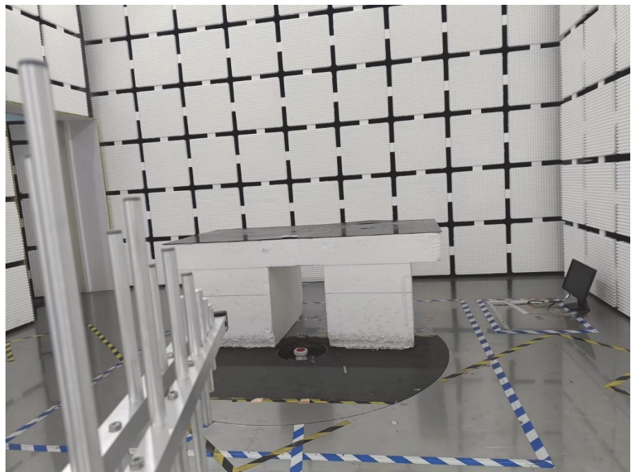
Radiation Emission Test Setup (30MHz to 1GHz)
