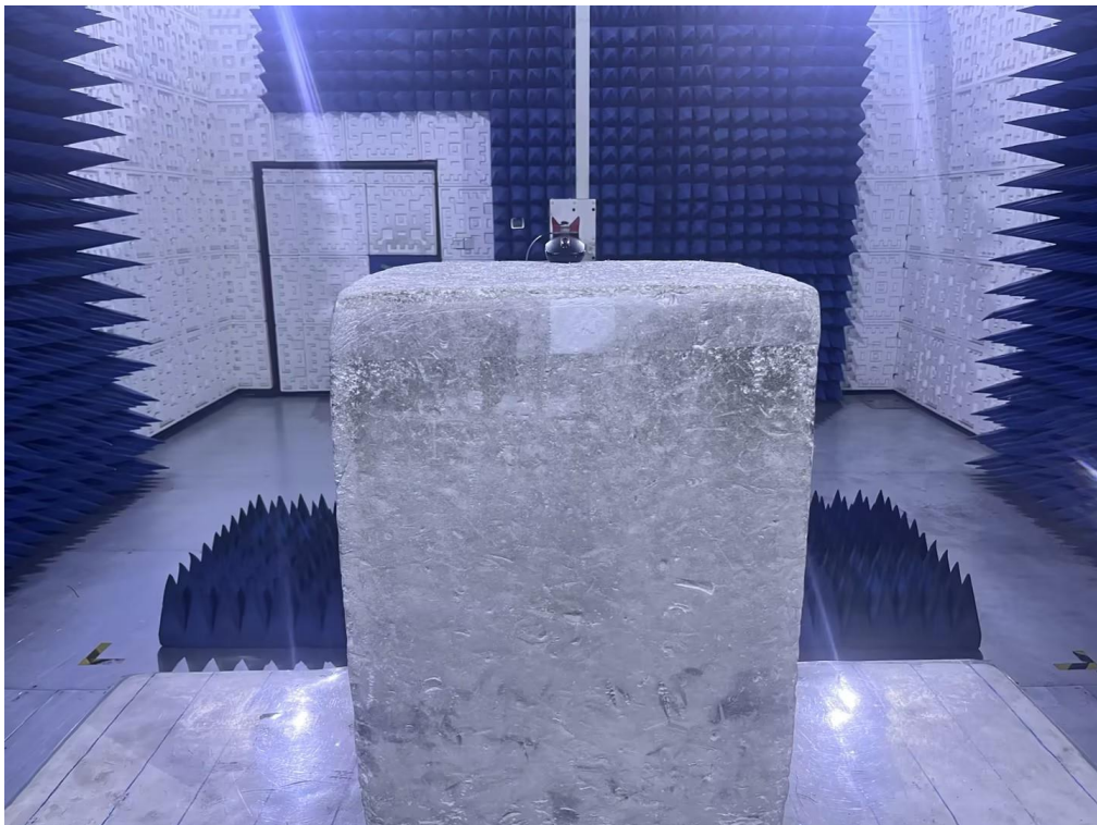
RADIATED EMISSION TEST SETUP ABOVE 1GHz
