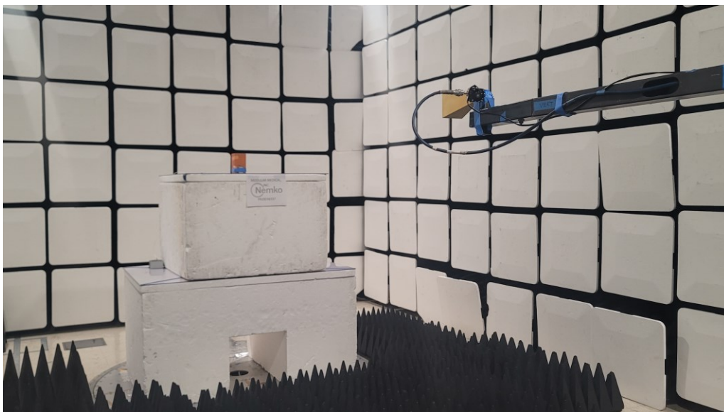
Figure 6 - Radiated emissions above 1 GHz (18 – 26.5 GHz), front view.
