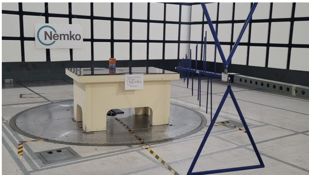
Figure 2 - Radiated emissions below 1 GHz (0.03 – 1 GHz), front view.
