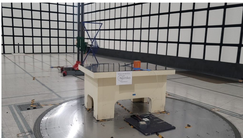
Figure 3 - Radiated emissions below 1 GHz (0.03 – 1 GHz), rear view.
