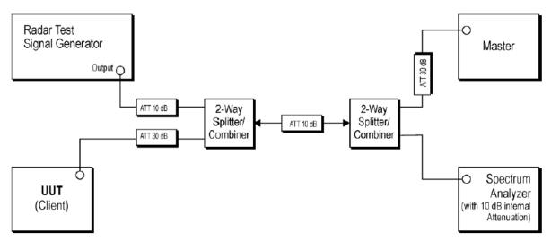
Radar Test Waveforms are injected into the Master.
