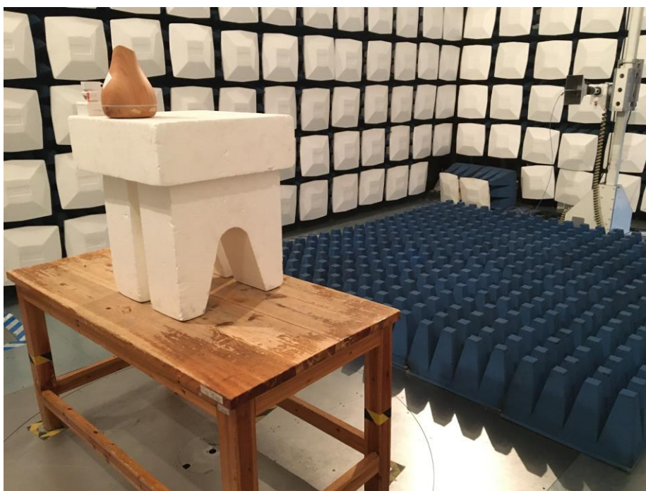
Test Setup For Radiated Emission (Above 1GHz)
