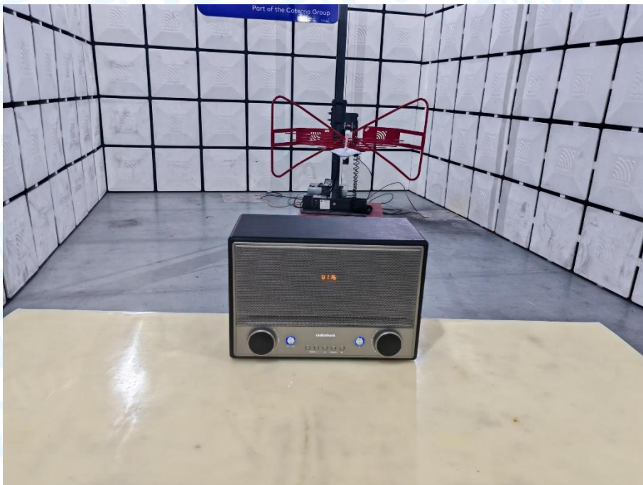
Photo of Setup for Radiated Emission (30MHz~1GHz)
