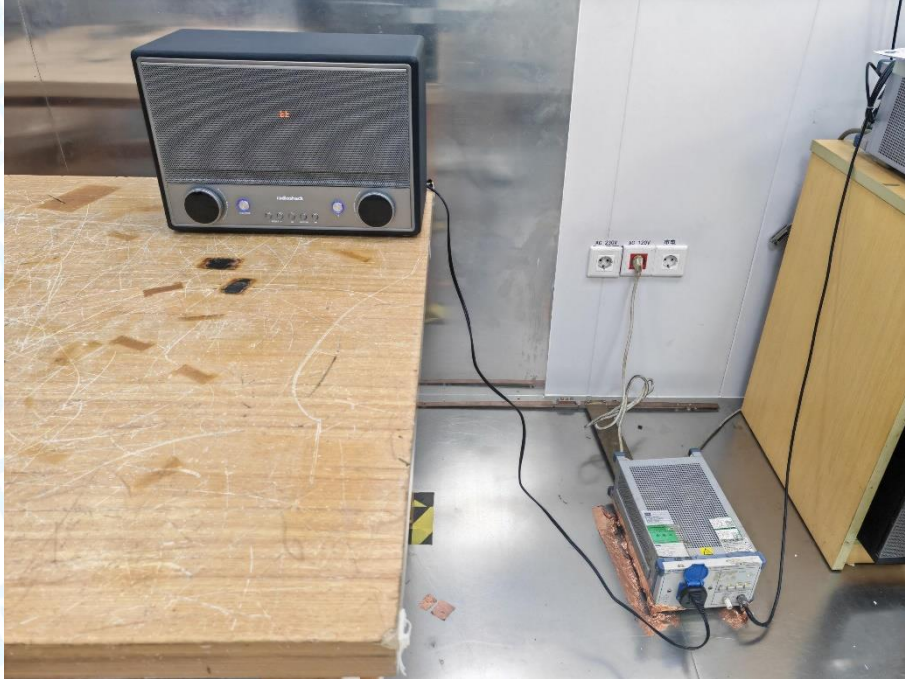
Photo of Setup for Radiated Emission (30MHz~1GHz)
