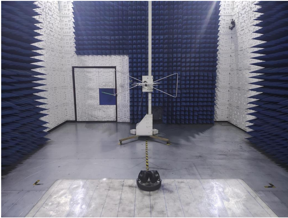
RADIATED EMISSION TEST SETUP ABOVE 1GHz
