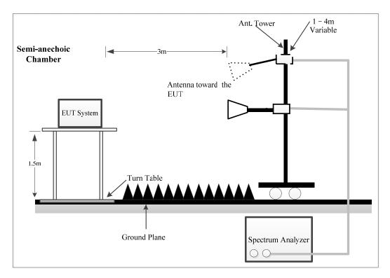
The radiated emissions were performed in the 3 meters distance, using the setup accordance with the ANSI C63.10-2013. The specification used was the FCC 15.209, and FCC 15.249 limits.
