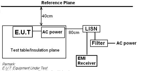
E.U.T. Equipment Under Test LISN: Line Impedence Stabilization Network Test table height=0.8m
