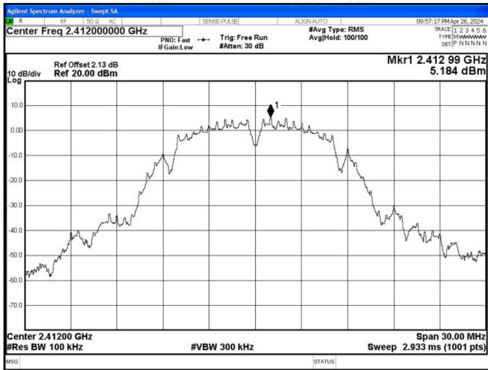
Tx. Spurious NVNT b 2412MHz Ant1 Emission
