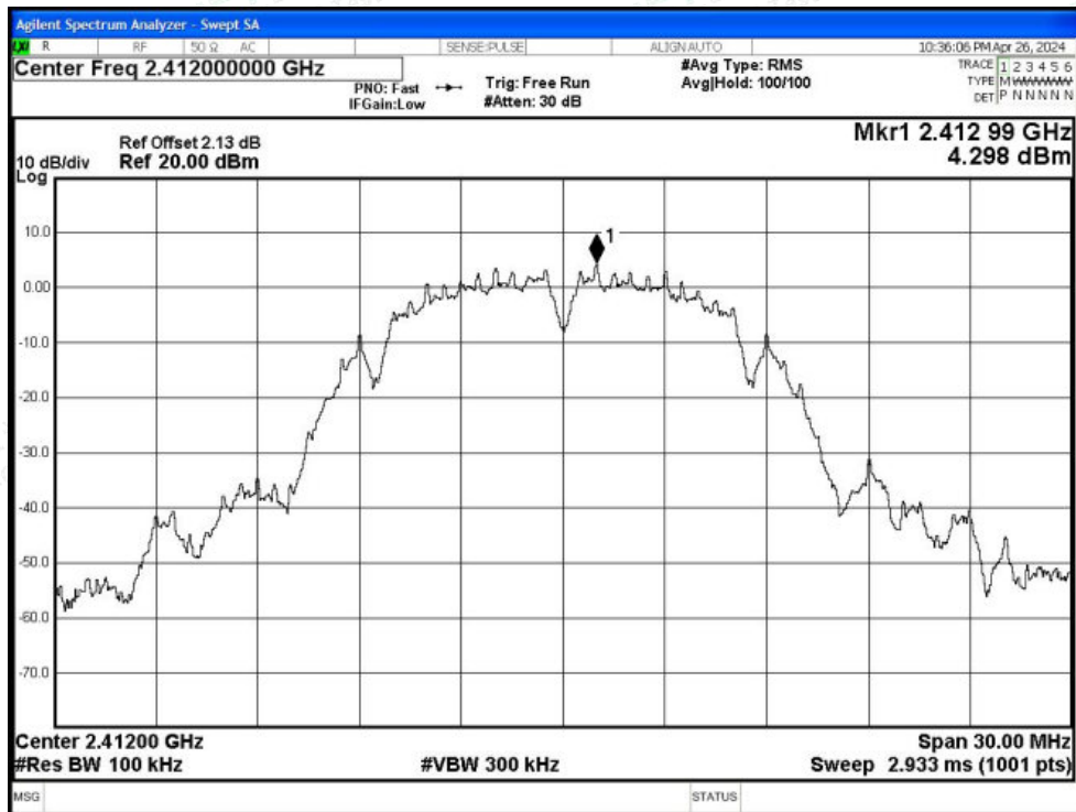
Band Edge NVNT b 2412MHz Ant2 Emission
