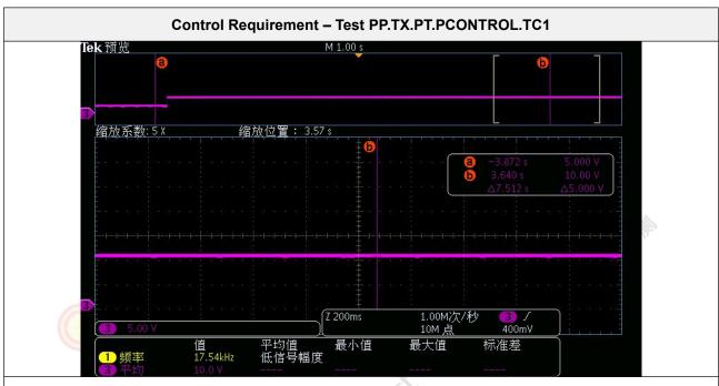
Test PP.TX.PT.PCONTROL.TC1: The measured rectified voltage was 10.00 V.
