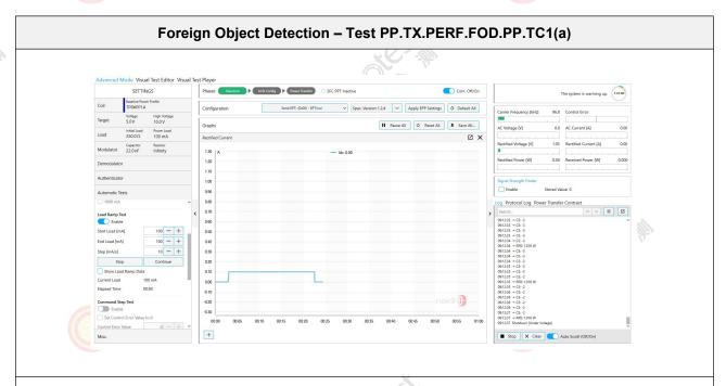
Test PP.TX.PERF.FOD.PP.TC1(a) (Foreign Object #1): The BSUT does not initiate power transfer.
