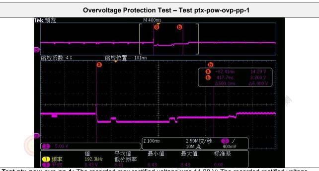
**Test ptx-pow-ovp-pp-1:** The recorded max rectified voltage was 14.20 V; The recorded rectified voltage was 8.20 V in between Packets from 500 ms after the load step until the end of the recording.
