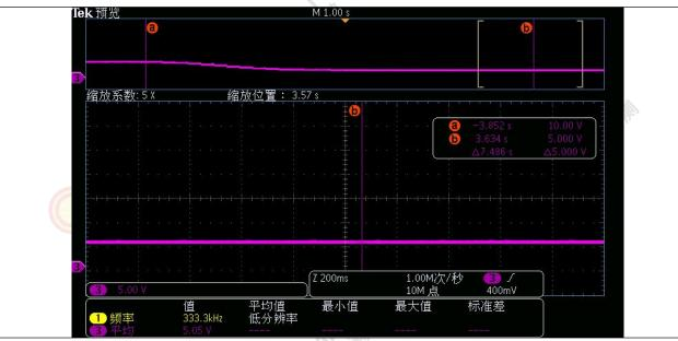
Test PP.TX.PT.PCONTROL.TC2: The measured rectified voltage was 5.05 V.
