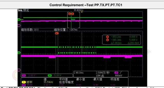
**Test PP.TX.PT.TC1:** The time that BSUT responds with an FSK Packet (PP\_TX) from the end of the Control Error Packet was 7.86 ms.
