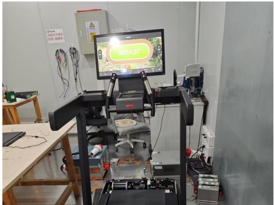
Conducted Emission Test Setup
