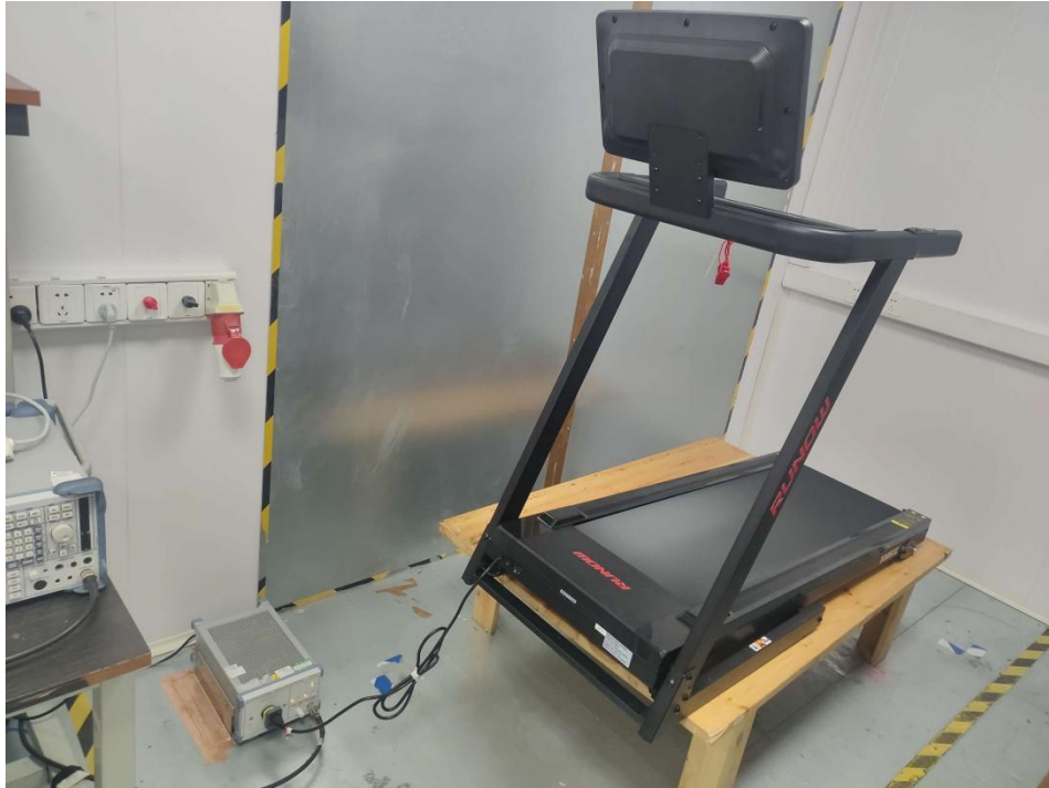
Conducted emissions at AC power line (150kHz-30MHz)
