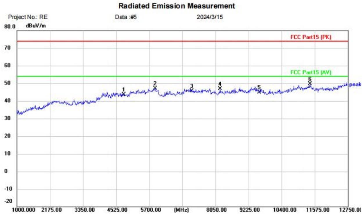
Site: Limit: FCC Part15 (PK) EUT: Electric treadmill M/N: 3305 Mode: TX-2402 Note: Polarization: **Horizontal** Power: Temperature: (C) Humidity: %RH
