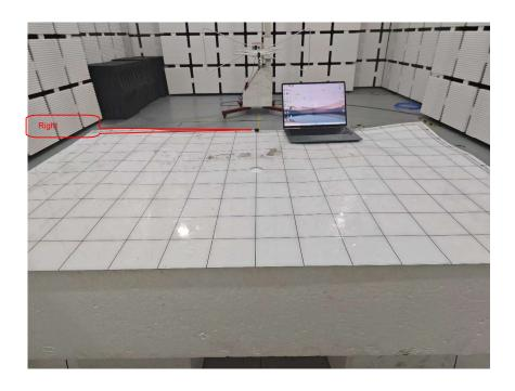
Set-up for Radiated Spurious Emission, Above 1GHz
