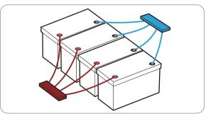
①Bus Bar: It can help ensure the input & output currents of each battery are balanced and improve the conversion efficiency of the input & output currents for the battery.
