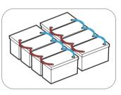
Connect the batteries in parallel.
