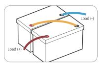
After series connection, the voltage of the battery system will be doubled according to the number of batteries vou connect.
