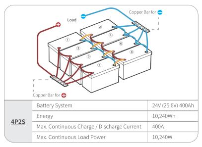
① As  $\bigcirc$  of ① / ③ / ⑤ / ⑦ is connected in series with  $\bigcirc$  of ② / ④ / ⑥ / ⑧, please do not connect  $\bigcirc$  of ① / ③ / ⑤ / ⑦ with  $\bigcirc$  of load or  $\bigcirc$  of ② / ④ / ⑥ / ⑧ with  $\bigcirc$  of load, otherwise the battery system will fail to connect in series.
