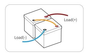
After series connection, the voltage of the battery system will be doubled according to the number of batteries you connect.
