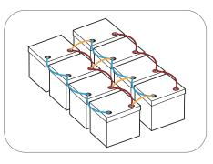
Connect the paralleled battery systems in series.
