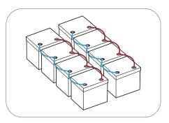
Connect the batteries in parallel.
