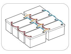
Connect the paralleled battery systems in series.
