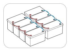
Connect the batteries in parallel.
