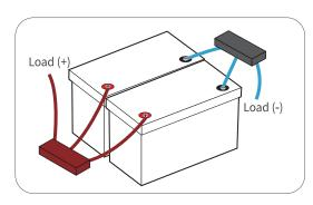
After parallel connection, the capacity of the battery system will be doubled according to the number of batteries you connect.
