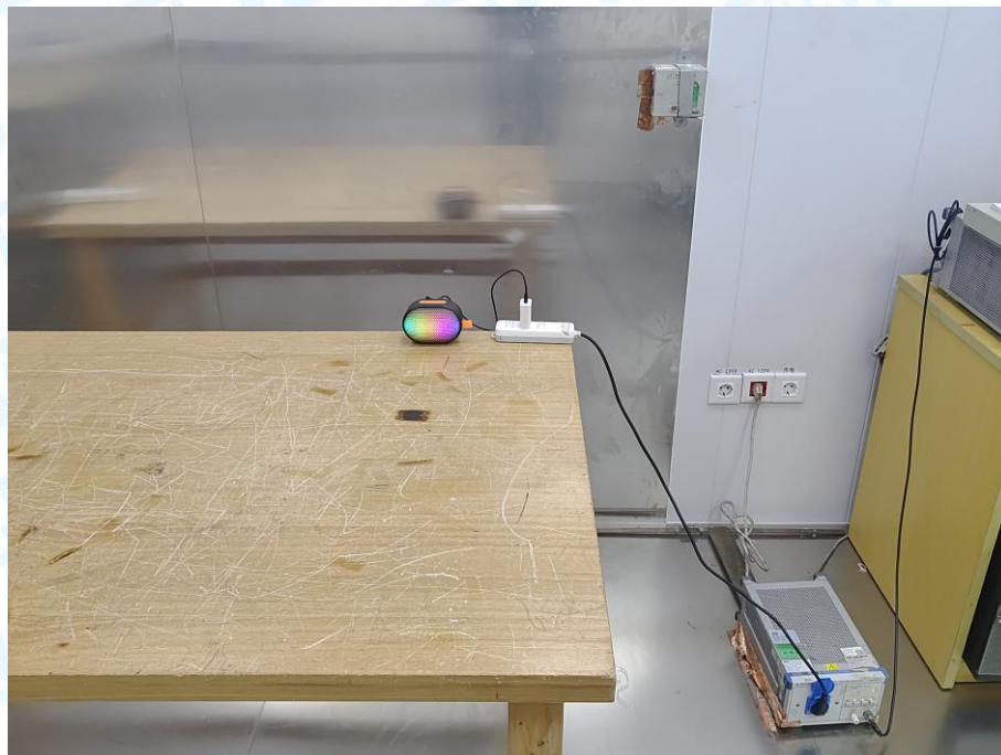
Photo of Setup for Conducted Emission
