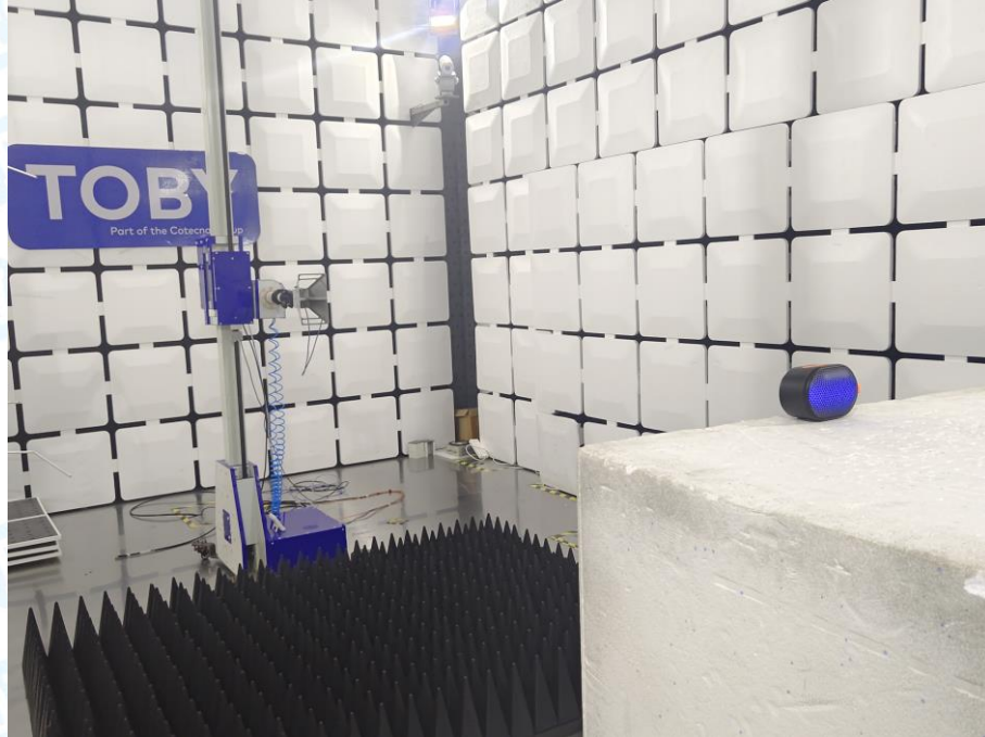
Photo of Setup for Conducted Emission
