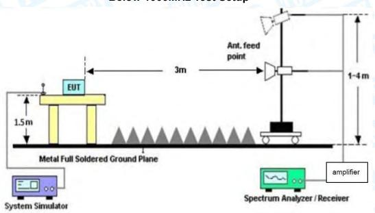
**Above 1GHz Test Setup**
