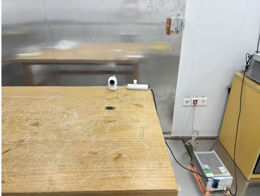
Photo of Setup for Radiated Emission (30MHz~1GHz)
